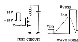
$$\begin{split} R_G &= 25~\Omega \\ V_{DD} &= 90~V,~L = 357~\mu H \end{split}$$
